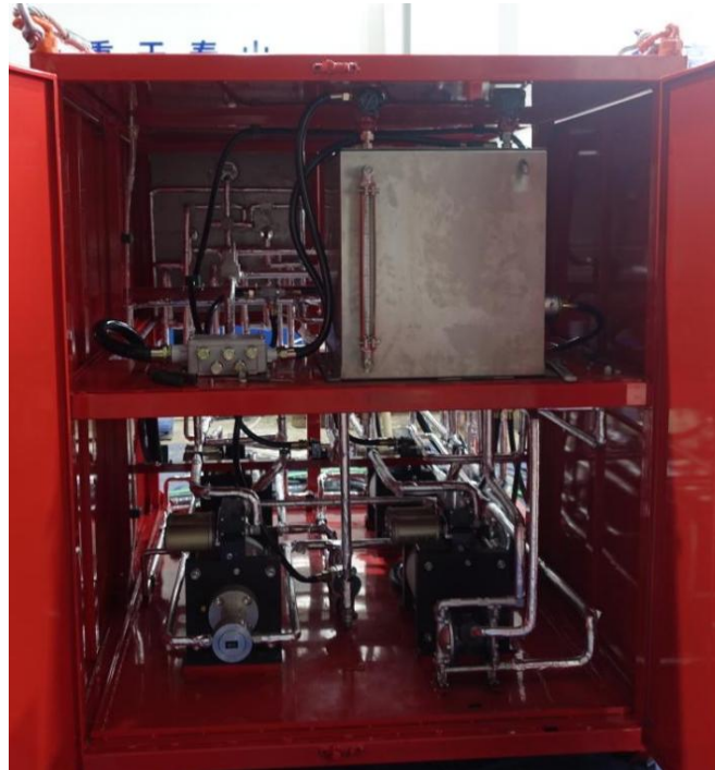
Figure 2.4 Chemical reagent injection skid
