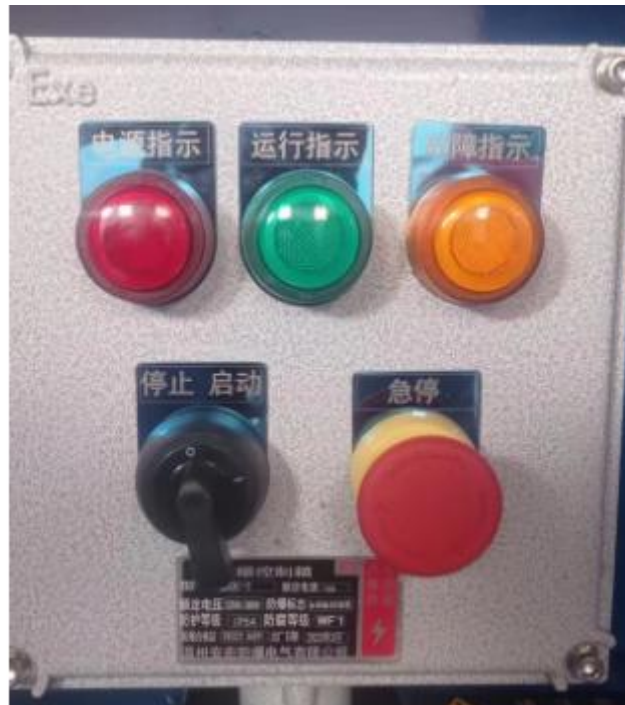
Figure 2.9 Manual operation panel layout
