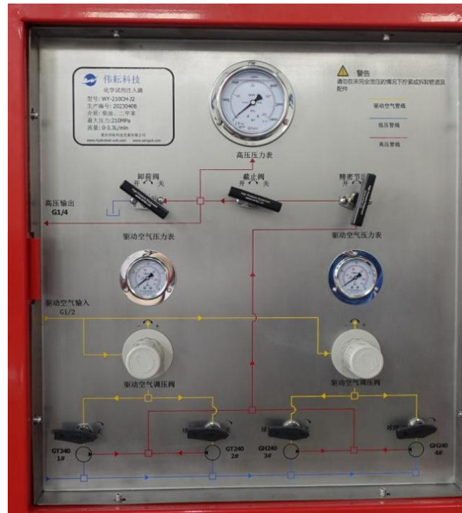
Figure 2.5 Manual operation panel layout
