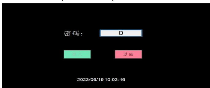
The password is a dynamic real-time date (for example, the date is June 1, 2023, and the password is 20230601)
