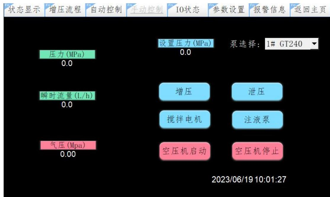
Boost: boosting according to the set pressure and the selected pump
